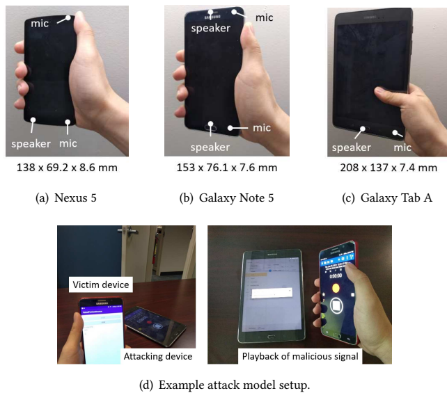
Figure 9: Experimental setup for evaluating EchoLock . (a) through (c) show example holding styles and devices specifications, (d) depicts evaluation of the adversary model.
